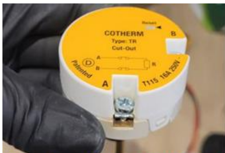
Figure 1: Immersion heater over-temperature cutout, with evidence of discolouration at the live terminal
