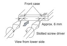
**b.** To open the case, pull up the front side from the bottom and unhook the tabs at the upper and lateral sides. Do not apply an excessive force when opening the front and rear sides of the case, as they are joined with connection bands.
