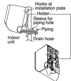
There is an option to use the holder at the rear of chassis to prop up the indoor unit as shown in the illustration for ease of installation. Push the holder back to original position before secure the indoor unit.
