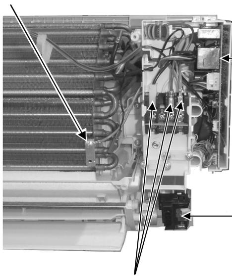
10. Pull out the Main Electronic Controller halfway.
