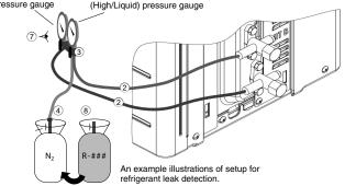
Step 2: Refrigerant leak detection through Electronic halogen leak detector and/or ultrasonic leak detector:
