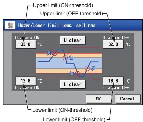
Note: To clear the ON- and OFF-thresholds for the upper limit temperatures, touch [U clear]. To clear the ON- and OFF-thresholds for the lower limit temperatures, touch [L clear].
