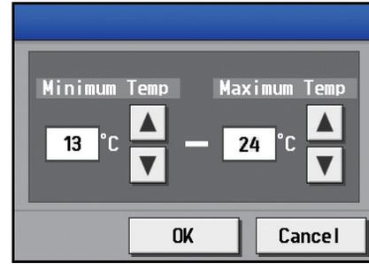
Note: The air conditioning units in the heating operation will stop and the set temperature will return to the original setting when the Setback Control period is over or the room temperature rises to the minimum temperature plus 3°C (6°F). Likewise, the air conditioning units in the cooling operation will stop and the set temperature will return to the original setting when the Setback Control period is over or the room temperature drops to the maximum temperature minus 3°C (6°F).
