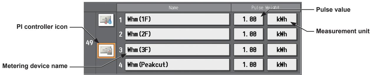
(1) Using the scroll bar, select the address to which the PI controller (PAC-YG60MCA) will be connected.
