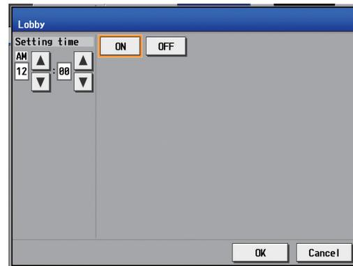
Note: When setting a schedule for a block or all groups, all operation modes are available for selection, but the available operation modes depend on the unit model. The units will not operate in the selected mode not supported by the units.
