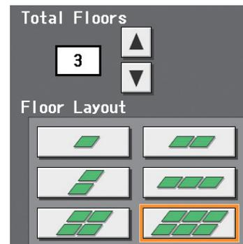
The display range of the area on the [Floor Layout] screen vary, depending on the selected floor layout.
