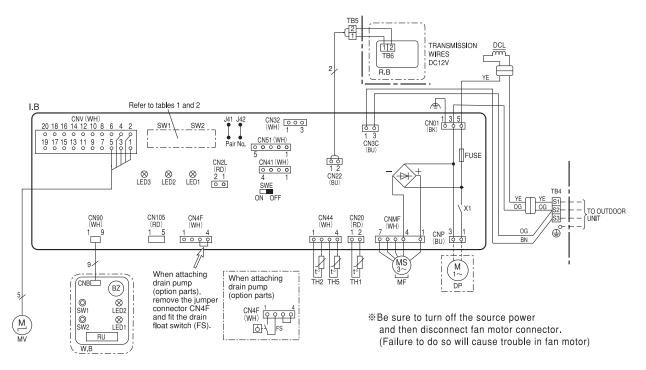
Notes: 1.Symbols used in wiring diagram above are, ooo:Connector, :Terminal (block).
