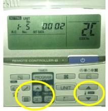
Press the SPANNER button to cancel detailed setting operation. Turn off power. Remove the BL sensor from its socket on the indoor PCB. Snip the Plug from this sensor ensuring there is 80mm of cable still connected to the plug. Tape up the wiring going to the sensor. This will not be needed.
