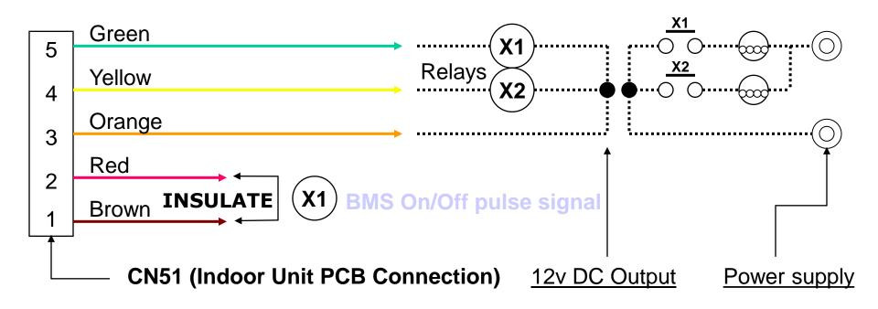
Pin 3 will give a permanent 12vDC Output. Pins 5 and 3 for Alarm Output Pins 4 and 3 for Run Output Note that colours above may change. Use pin numbers for accuracy. X1 and X2 – field supply relays
