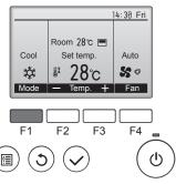
Press F1 button to go through the operation modes in the order of "Cool", "Dry", and "Fan". Select the desired operation mode.
