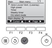
③ Press F1 or F2 button to go through the vane setting options: "Auto", "Step 1", "Step 2", "Step 3", "Step 4", "Step 5" and "Swing", and select the desired setting.
