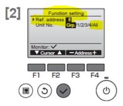
You now need to select Mode No. 1 & Setting Data 2 to activate Auto Restart After Power Failure. If you would like to turn off Auto Restart, please select Setting Data 1 and tick to confirm.
