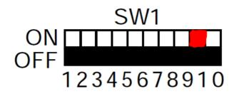
When in the ON position prior to power being taken away, the unit will resume the operation it was in when power is restored.
