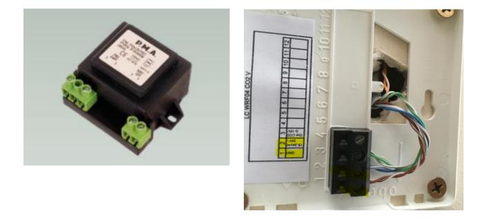
Connecting the postive + to terminal 2 of the Co2 Sensor & the negative – wire to terminal 1 (GND).
