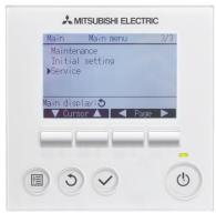
In the main menu screen move the cursor using F1/F2 to Service option and press
