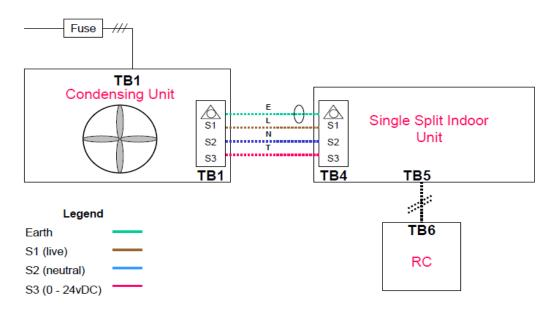
As an alternative, a separate terminal block can be purchased to allow you to provide a separate 240vAC supply to the indoor unit. This plugs into **CN01** on the Indoor PCB.
