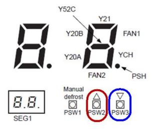
To start the viewing system information from the outdoor unit, hold the **PSW2** button for 3 seconds, the display should light up or change from current display.
