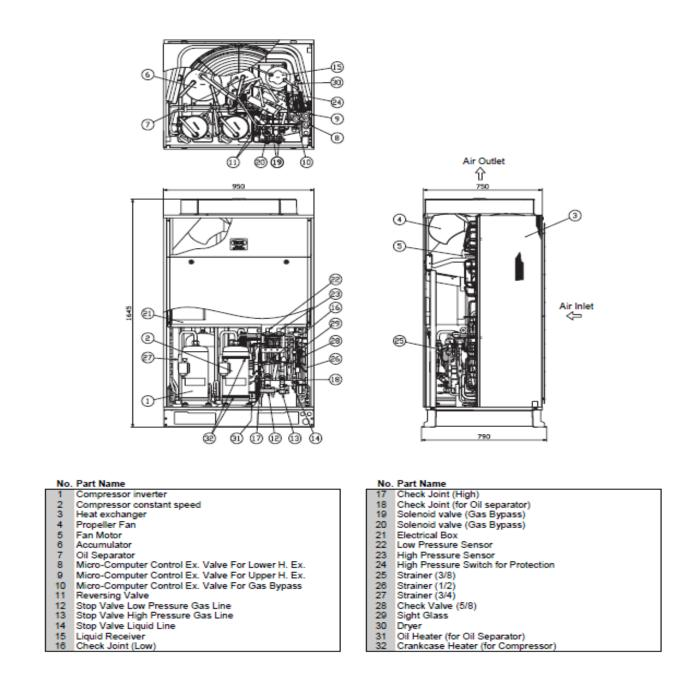
The oil can be checked by removing a sample from the  $\frac{1}{4}$ " port at the bottom of the **Oil Separator** (Item 7) & the **Check Joint** (for the Oil Separator item 18). If there is pressure in the system the oil will be pushed out through the  $\frac{1}{4}$ " line, and to recharge it use the same port by using an oil hand pump.
