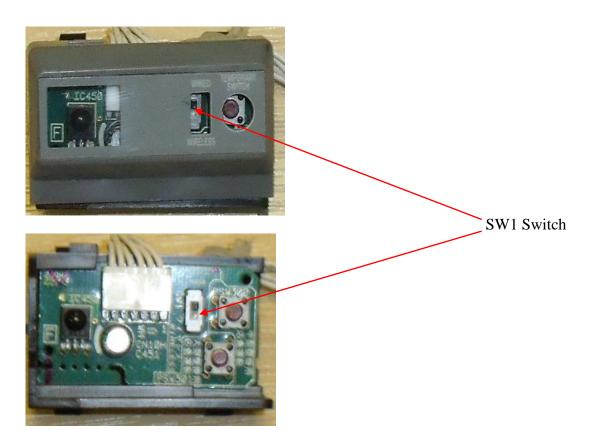
If this is not done, when you turn on the system the hard wired controller will not operate and. The controller will show a display but will not operate the unit.
