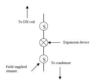
For applications between 8HP and 10HP you will need two valve kits coupled to a field supplied T-Joint. This will be ONE PANEL, TWO VALVES
