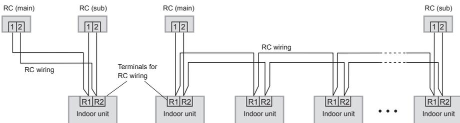
**EN** \*Remote controllers can be connected to any indoor unit for operation.
