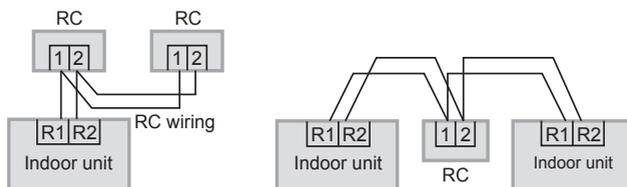
**EN When setting both the main and sub remote controllers**
