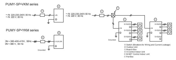
■ Schematic Drawing of Wiring: When using a Branch Box and M-NET control indoor unit (example)
