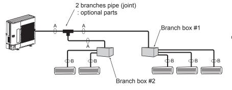
Installation procedure (2 branch pipe (joint))
