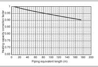
Figure 6 Correction of refrigerant piping length
