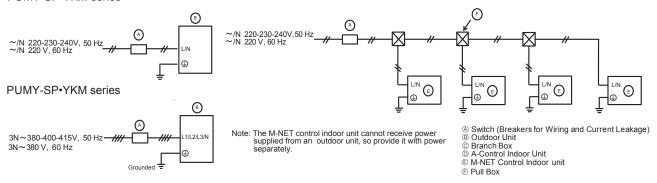
■ Schematic Drawing of Wiring: When using a Branch Box (example)
