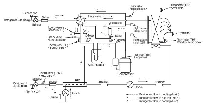
Capillary tube for oil separator :  $\phi$ 2.5 ×  $\phi$ 0.6 × L1000
