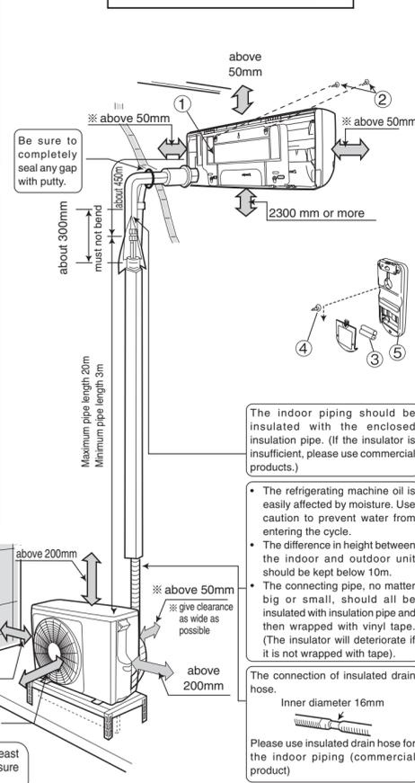
The indoor piping should be insulated with the enclosed insulation pipe. (If the insulator is insufficient, please use commercial products.)
