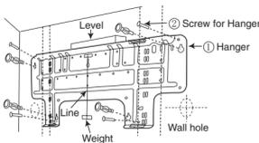
Screw the hanger at the positions possibly near the upper and lower hooks where the indoor unit is hung. Use 4 or more screws to fix the hanger.
