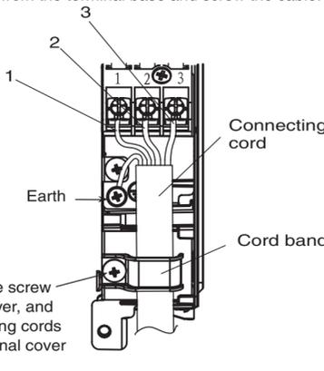
After remove the screw and terminal cover, and put the connecting cords and fix the terminal cover with screw.
