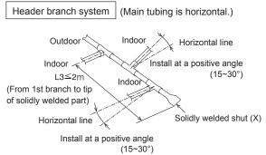
• Be sure to solidly weld shut the T-joint end (marked by X in the figure). In addition, pay attention to the insertion depth of each connected tube so that the flow of refrigerant within the T-joint is not impeded.
