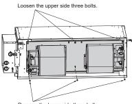
Remove the lower side three bolts.
