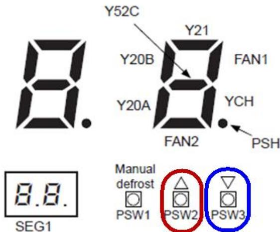
To start the viewing system information from the outdoor unit, hold the **PSW2** button for 3 seconds, the display should light up or change from current display.
