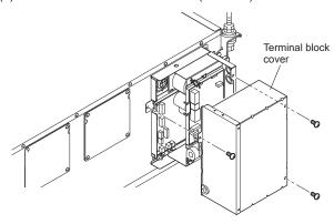
(2) Connecting the power supply cable and transmission cable. Pass the Power supply cable through the bush\* and connect to the TM1 terminal block using the round terminals. Connect the ground wire to the ground terminal and secure tightening the bush. (\* Use an item that can firmly secure the cable such as a PG connector.)
