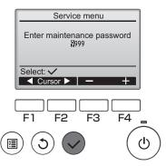
Enter maintenance password "0000" is displayed. Enter the initial password "9999" and press the SELECT button.
