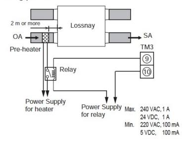
It is then necessary to program the PZ-62DR-E to implement the pre-heater output setting.
