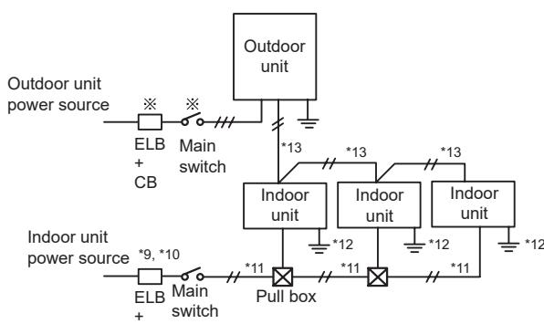
**Example of wiring connection Heat recovery system**
