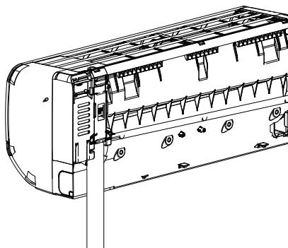
**For installing securing plate (only 2.0 to 4.0 HP)**
