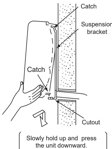
When removing the indoor unit, push up the "PUSH" part on the bottom side and pull the unit to the front side. Therefore, the catches are released from the suspension bracket.
