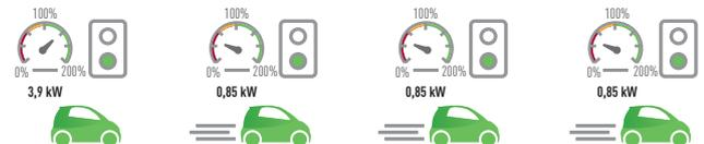
**NO INVERTER** Slow to start. Takes longer to reach the temperature set point. The temperature oscillates between the two extremes and never stabilises. The temperature falls and then rises quickly, leading to a consumption peak.
