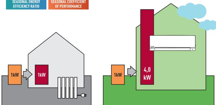
\*Heat pump vs Electrical Heaters. Heat pump is using free energy existing on the air, that is why by using 1kW of electrical energy, KIT-RE9/12-QKE supplies 4kW of heating energy.
