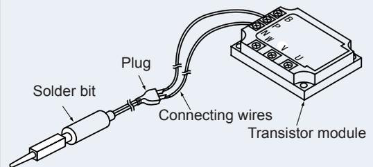
**Transistor module checking procedure**
