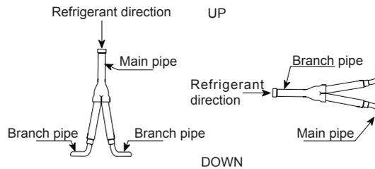
4 Correct position of Triple/Quad distributor.
