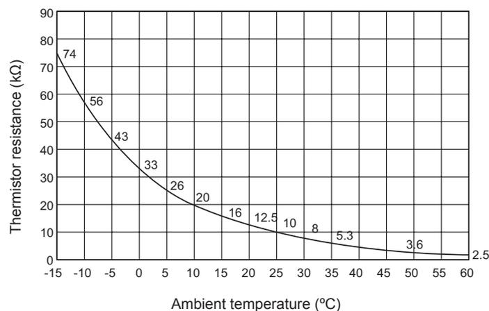
Ambient and evaporating temperature thermistor characteristics for RASC unit
