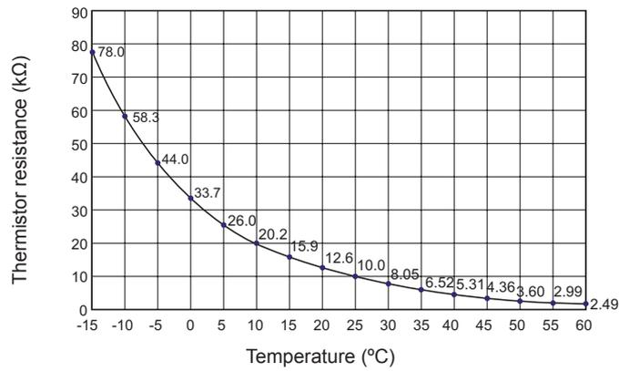
◆ **Thermistor for inverter fin temperature (THMI)**
