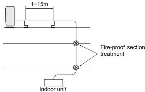
Do not fix the refrigerant piping directly with the metal fittings (The refrigerant piping may expand and contract).
