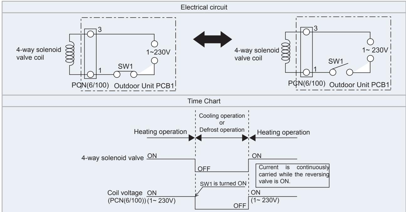
**Bistable solenoid operation type (pulse-activated)**
