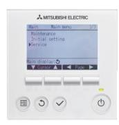
In the Main Menu screen move the cursor to the **SERVICE** option and press  $\checkmark$
