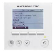
Move the cursor to the FUNCTION SETTING option and press  $\checkmark$
