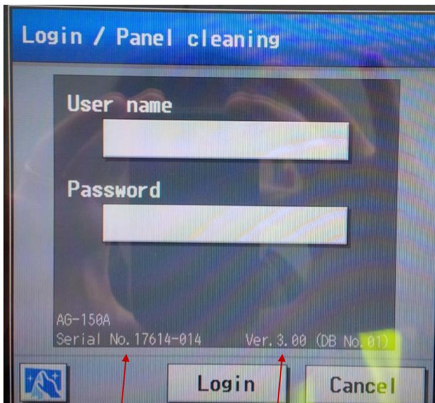
If you are in the normal monitor/operation screen, press the spanner icon in the top right hand corner to bring up the log in screen above.
