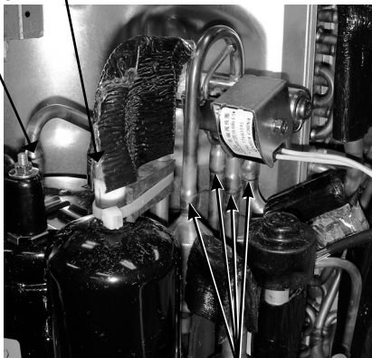
Brazed parts of 4-way valve
