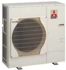
Heat energy from the outside air and a little mains electricity is used by the Air Source Heat Pump to heat refrigerant to a high temperature. This heat is then transferred to water which flows into your home for central heating and also for domestic hot water for baths etc. The way the heat pump works is similar to a refrigerator in reverse.
