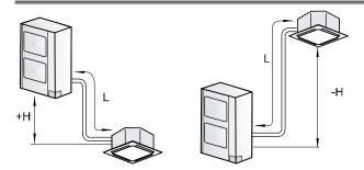
The correction factor is based on the equivalent piping length in meters (EL) and the height between outdoor and indoor units in meters (H).
